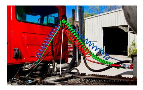
The rod on the MAXXDuty pogo is made of fiberglass and eliminates the need for an internal spring. It has undergone extensive testing (over a half million cycles without signs of failure) and over a year of field trials in the harshest conditions with no signs of wear – that's 10 times longer than traditional pogos! Plus, the MAXXDuty Pogo features a nylon polymer all-in-one hoop that allows for total flexibility in managing critical air, electrical and hydraulic lines.
