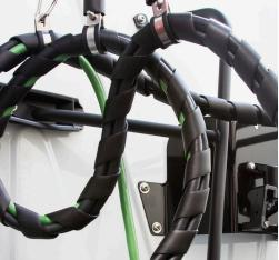
**TECH TIP:** Avoid damage and CSA violations by utilizing multiple tender springs to hang your wrapped lines instead of just one. This reduces stress on the springs so they won't stretch out and allow your lines to drag on the deck plate.
