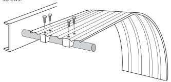
5. On the underside of the fender, loosely assemble the clamping plates to the ISO-BLOX with the  $5/16'' \times 3/4''$  hex head bolts and lock washers.
