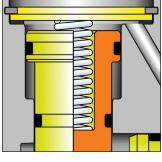
By design, the spring brakes will retain the maximum pressure delivered by the compressor, until the supply gladhand pressure drops to about 35 psi. The effective area of the shuttle at gladhand pressure is about 3 times that of the area exposed to spring brake pressure.
