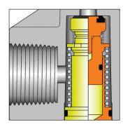
PRESSURE PROTECTION: When the supply line pressure exceeds 85 psi. the piston shifts down to allow flow to the tank. The check valve retains tank pressure when the gladhand is vented.
