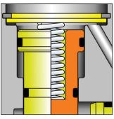
**RESERVOIR SENSOR:** The reservoir sensor section measures the tank pressure and prevents air from flowing into the spring brakes before service braking capability builds in the system.
