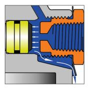
**VENTING ANTI-COMPOUNDING: When** the spring brakes are on, the control line is vented to atmosphere. This prevents false release of spring brakes on doubles and ejects fluids trapped in control lines.
