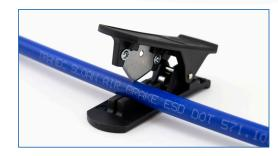
QUICK TIP: To ensure your PTC fittings form a tight seal that's free from leaks, always cut your air brake tubing squarely and with a clean edge. Using a tube cutter (like p/n 451100 pictured above) is the easiest way to do this!
