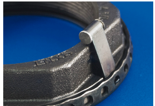
Locking clip detail of Trailer Axle Nut #MF111077
