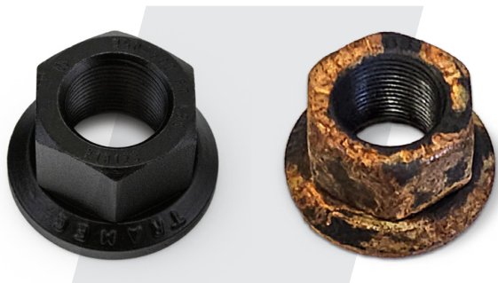
Tramec Wheel Nut (Left) and the Competition (Right) after 240 hours of salt spray testing
