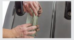
2. Remove white backing tape to expose the sticky resin. Apply patch to repair area with sticky side down and press firmly to make sure the patch seals the entire area.
