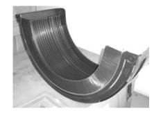
3) When the brush is located in the channel, check to make sure that it is spaced evenly. Then push into place using a large flat blade screwdriver or similar tool. Starting at the center of the brush, push on the edge of the metal backing. Continue to work towards the ends.
