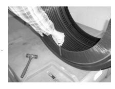
4) When the brush is in place, fasten it through the holes in the mounting tabs with the provided self-taping screws. Be careful not to over tighten!
