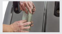
Remove white backing tape to expose the sticky resin. Apply patch to repair area with sticky side down and press firmly to make sure the patch seals the entire area.
