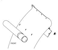
Install the support strap on the back side of the fender using (3) 3/8-16 serrated flange nuts. Torque to 23 ft-lbs.
