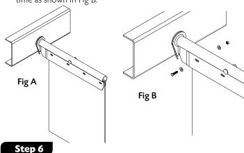
Install the first three bolts and tighten by hand.
