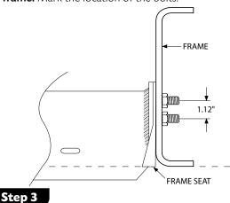
Drill 17/32" clearance holes for the bolts and mount FB bracket as shown.
