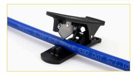
QUICK TIP: To ensure your PTC fittings form a tight seal that's free from leaks, always cut your air brake tubing squarely and with a clean edge. Using a tube cutter (like p/n 451100 pictured above) is the easiest way to do this!
