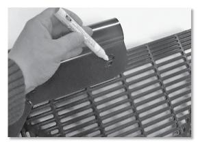
**5.** Remove the AeroFlap<sup>®</sup> from the bracket, place on a solid surface and use a drill to make the necessary holes.
