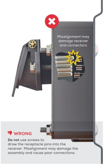
1) The application of a non-conductive (dielectric) grease, per TMC recommended practice RP-155, to the rear pins of the receptacle and the receiver sockets can **reduce installation force** and **increase life** of the connector.
