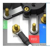
• Tighten nuts securely against the harness ring terminals, using 15 to 20 lb-in torque.
