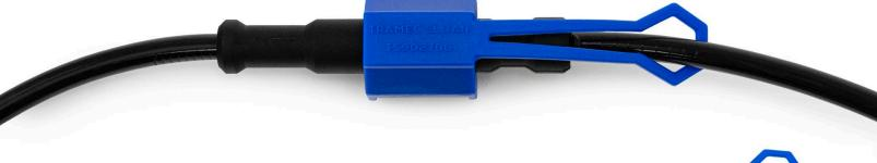
Tramec Sloan's teathered ABS Sensor Lock firmly secures the extension cable to the ABS sensor, ensuring a dependable and uninterrupted connection. Engineered with precision, it eliminates the risk of loose connections that could lead to sensor malfunctions or operational interruptions, providing peace of mind on the road.
